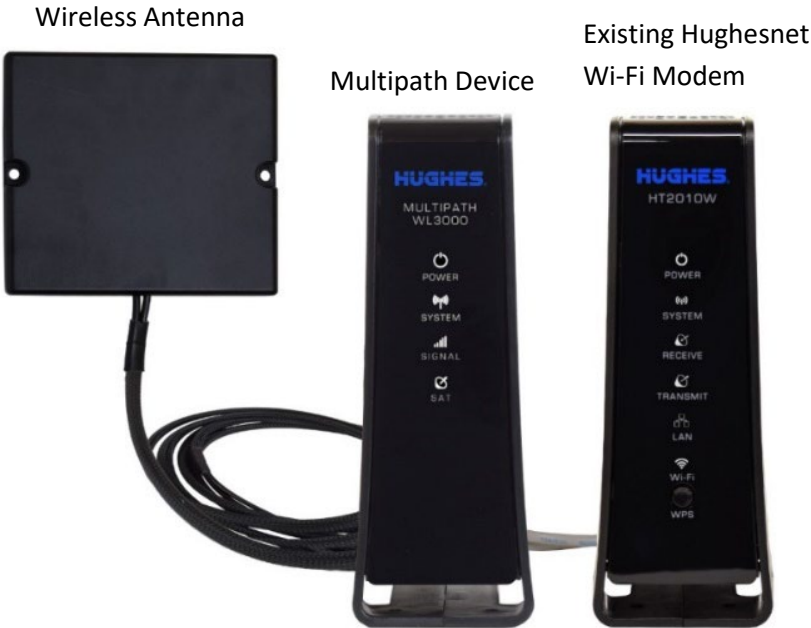
Figure 1: Connected Antenna, Multipath Device, and Hughesnet Wi-Fi Modem
