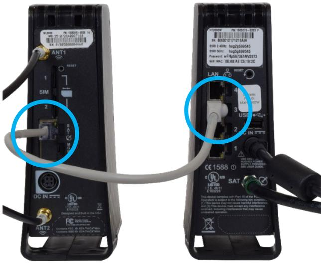
Figure 7: Multipath Device Ethernet cable connection
