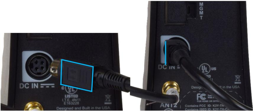
Figure 9: Aligning the power adapter connector
