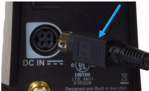
Figure 5: Locking mechanism
